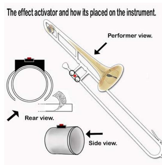
Figure 1. Effect activator here seen from three angles. Rear view shows how it's attached to the trombone with Velcro.
